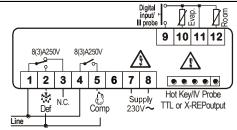
9-40Vdc supply: connect to the terminals 7 and 8. 12Vac/dc supply: connect to the terminals 7 and 8. 24Vac/dc supply: connect to the terminals 7 and 8. 120Vac supply: connect to the terminals 7 and 8.
