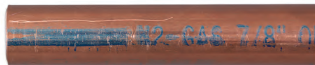
Figure 2 - Copper tube with "bad" surface scratch.
