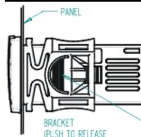
Instrument XR64CX shall be mounted on vertical panel, in a 29x71 mm hole, and fixed using the special bracket supplied.
