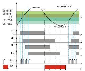
This draw highlights the doF time: the loads are in fact turned off only when the doF time is over.
