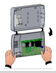
Make all the electrical connections with reference to the annexed diagrams for the respective model (see the tables in the ANNEXES). To carry out the electrical connections reliably and maintain the degree of protection of the box, we recommend using suitable cable glands and / or pipe clamps to tightly seal all the wiring.
