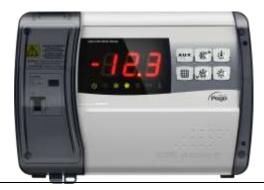
Be sure not to tighten the closing screws excessively as this could cause the box to become deformed and jeopardise its correct functioning and tactile effect of the keyboard on the panel; do not exceed 1 newton meter of torque. Install protection devices against power surges for short-circuits, in order to avoid damage to the device on all of the loads connected to the electronic controller ECP202 EXPERT 2EV.
