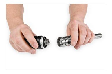
Separate the electronic part from the mechanical part.
