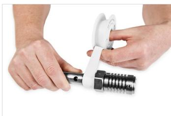
Apply Teflon or liquid gasket on sensors with a conical thread. For other thread types, solid gasket is used.
