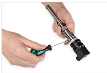
Loosen the 2 set screws that attach the electronic part to the mechanical part.
